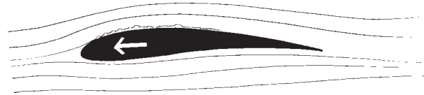
Fig. 12. The blade is relatively thick and the water does not have time to come around the blade. Bubbles are formed, in this case on the suction side.
