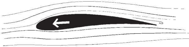
Fig. 11. The water flows evenly around the blade without bubbles.
