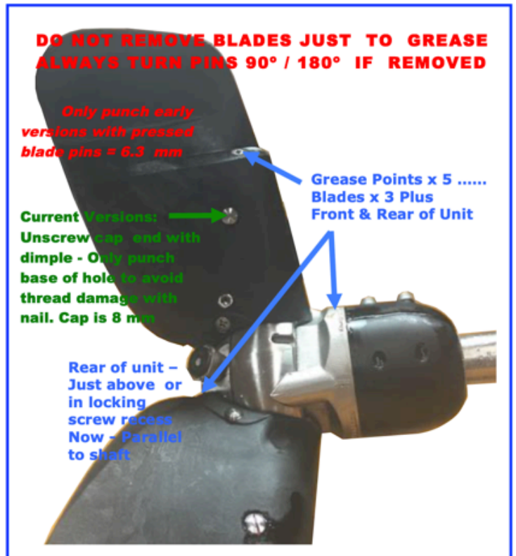
WEB PAGE ON BLADE MOUNTING COVERS LATER PIN VERSIONS WITH THREADED CAPS IN DETAIL .....
