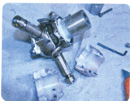
14. The spider in place. Note that there is no grease where the nose cone fits. A good grip is needed.
