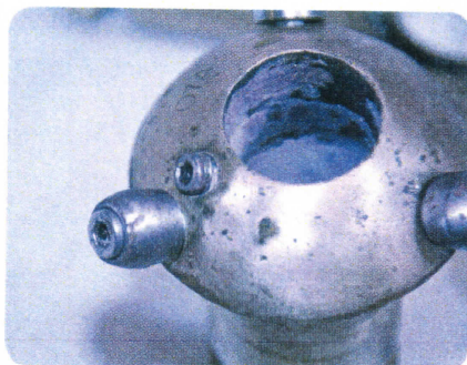
10. The only other parts for removal are the reversing cones.
