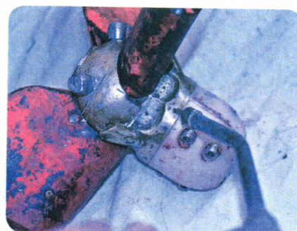
21. Don't forget the locking bolt on the spider.
