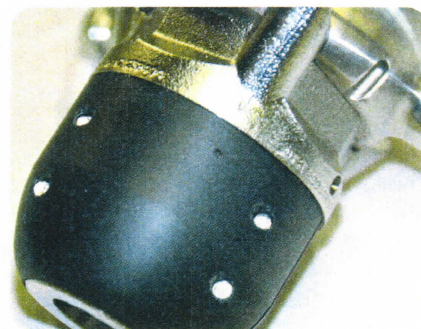
18. The nose cone is also marked for correct positioning.
