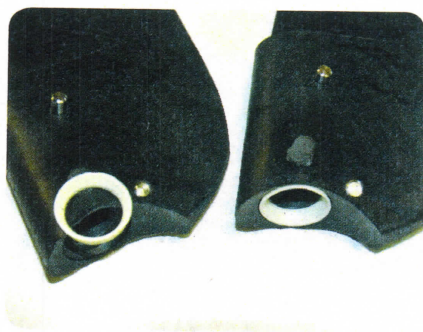
19. New model blades are fitted with improved seals.
