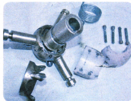
6. There are two set of slots in the hub. They dictate which way the propeller rotates so care is needed.
