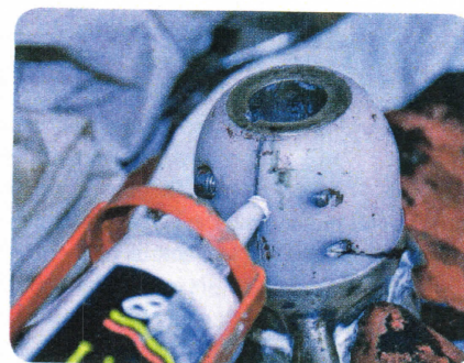
26. Sealant around the nose cone helps to seal the unit. New KiwiProps have this done in a special process at the factory.
