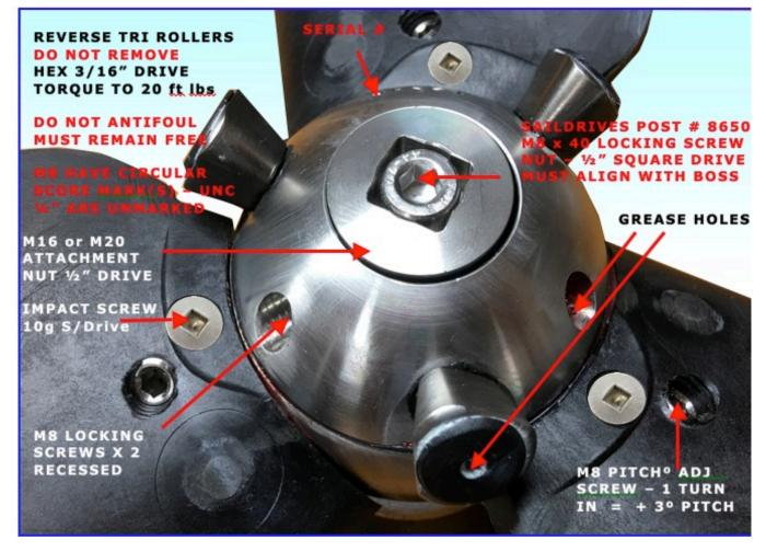
APPLY Loctite<sup>™</sup> or equivalent to the M16 or M20 NUT & M8 x 45 Cap screw on all Saildrives. Any Medium or Strong grade is appropriate. Its presence is more important than grade.
