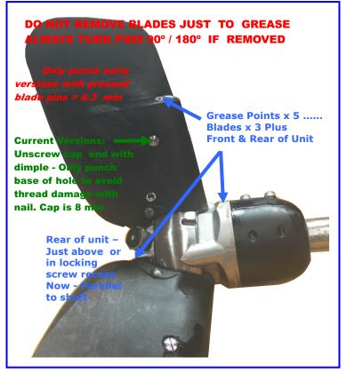
Refer to LUBRICATION and GREASING WEB PAGE ON BLADE MOUNTING COVERS LATER PIN VERSIONS WITH THREADED CAPS IN DETAIL .......
