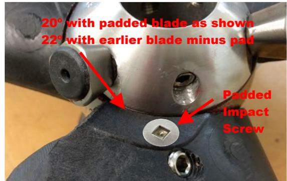
**IMPORTANT:** To avoid damaging the blade roots in reverse by exceeding the designed pitch settings when increasing the pitch, first lock the propeller by engaging ahead with the engine stopped. Rotate the propeller by hand into the reverse position against the spring, and then only increase the pitch until the blade comes up against the reversing rollers. *With Triangular rollers – turn the roller to contact the blade with a rounded section between the flats.*
