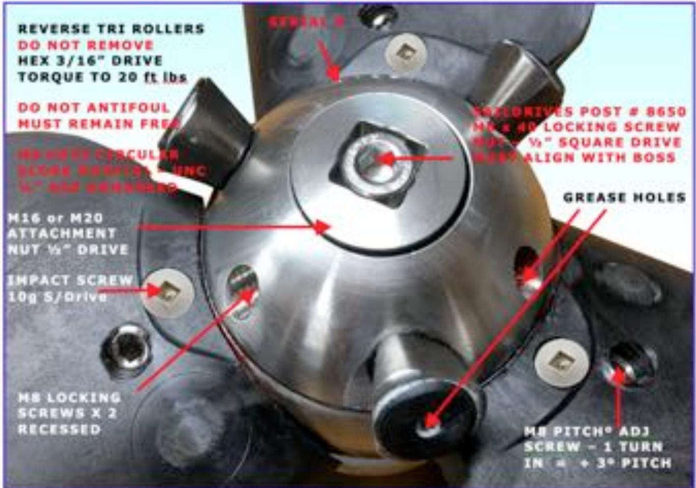
**APPLY Loctite™ or equivalent to the M16 or M20 NUT & M8 x 45 SCREW on all Saildrives. Any Medium or Strong grade is appropriate. It's presence is more important than grade.**
