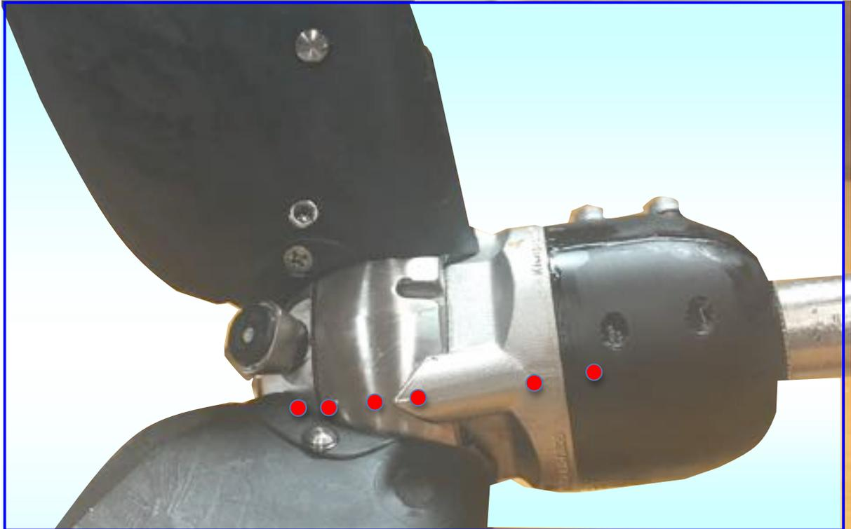
**WARNING:** Customers are strongly advised not to attempt to disassemble the unit unless this becomes absolutely essential. Re-assembly of all the components coupled with the need to ensure sealant is inserted into the nose cone whilst at the same time preloading the internal torsion spring makes for a tricky operation, particularly if no stub shaft is available to hold the unit whilst these operations are completed.
